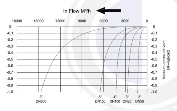
Fox ™ automatic air flowing out capacity, at high pressure, by size:
